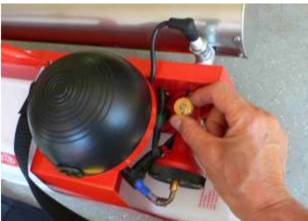
After the engine has started and warmed up readjust the adjustable screw...
