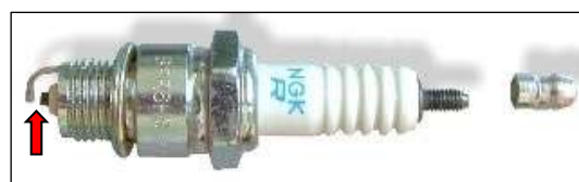
Space between electrodes : 1,5 – 2,0 mm
